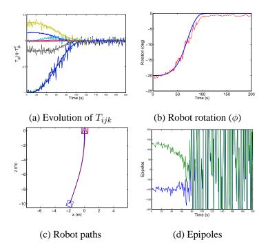
Fig. 7. Simulations with (thin line) and without (thick line) image noise of  $\sigma = 1$  pixel. The initial location is  $(-2, -10, -20^{\circ})$ . (d) Estimation of the epipoles to show the short baseline problem.
