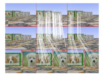
Fig. 5. Examples of images taken from the virtual scene. First row is the initial image, second row is a current image taken during the navigation and third row is the target image. Second column shows the SIFT matches between initial-current and current-target images. Third column shows the matches remaining across the three views after the robust computation of the trifocal tensor. Video attachments show the complete sequence of two simulations (videos 1 and 2).
