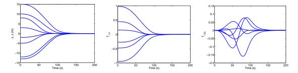
Fig. 3. Examples of several robot motions starting from different locations showing the evolution of x and z coordinates (left). For these different motions, we show the evolution of  $T_{111}$ , selected for the control (middle) and  $T_{133}$ , not used in the control (right).
