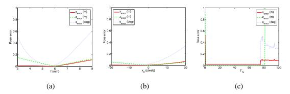
Fig. 8. Final location error in  $(x, z, \phi)$  varying the camera calibration parameters: (a) focal length and (b) principal point coordinates. (c) Final location error as a function of  $T'_N$ .
