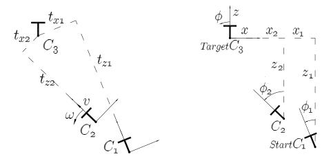
Fig. 2. Local coordinate systems (left) and global reference system (right) defined on the optical center of the cameras  $C_1$ ,  $C_2$  and  $C_3$ .
