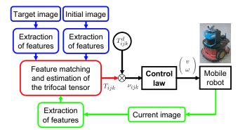
Fig. 1. Diagram of the trifocal tensor-based control loop.
